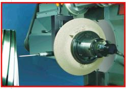
The working principle of this machine is form grinding. The profile of the grinding wheel is modified via on an on-board wheel dressing system and software package designed with a graphical interface to simplify complex profiling requirements.
