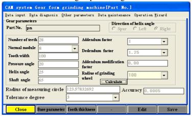
• Profile computing module for grinding wheel – Profile and Lead modification. This module serves to gather data in order to generate the correct wheel profile through an editable series of dressing cycles using the on-board dressing wheel system. Based on data entered about the workpiece and special requirements on gears to be machined; including profile, lead modification and fillet curve parameters, the profile of the grinding wheel can be automatically computed to meet the task at hand.
