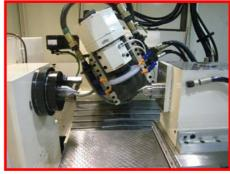
The working principle of this machine is form grinding. The profile of the grinding wheel is modified via on an on-board wheel dressing system utilizing a diamond
