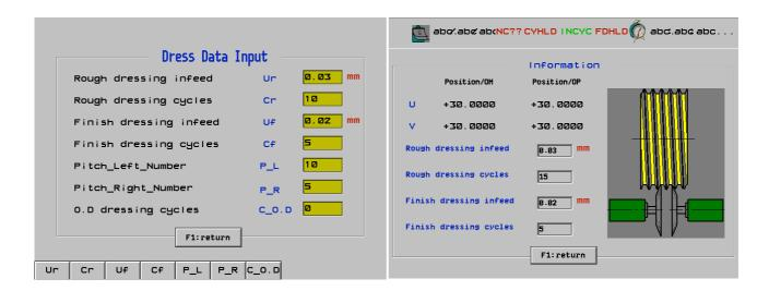
• Conversational Control Design. The G code will be automatically created based on the gear processing and grinding parameters entered by the user. In addition, the customers can even directly use and upload straight G code if desired.
